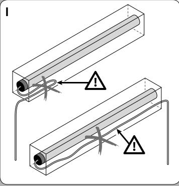
**CAUTION!** - The smaller cables must be handled carefully because they contain very thin wires that could be damaged.
