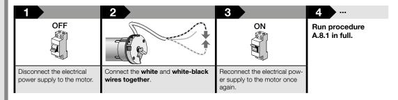
A.8.2.B - Procedure run with a transmitter that has not yet been memorised and the limit switch adjustment buttons on the motor head
