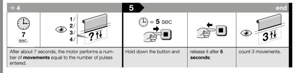
(\*) – IMPORTANT – After having programmed the option, or following the return of power after a blackout, 2 full manoeuvre cycles must be carried out straight away (Up and Down = 1 cycle) to activate the function. During this movement, the motor maps the instantaneous load along its travel and automatically sets the maximum sensitivity available with the awning in question.
